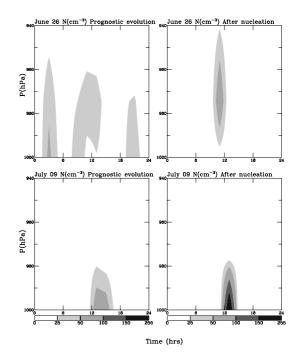
**Figure 6.** Time-pressure plot of the ECHAM simulation of cloud droplet number concentration (N) that shows the differences in N when N is treated prognostically and when N is calculated right after nucleation for the clean (26 June) and the polluted case (9 July).
